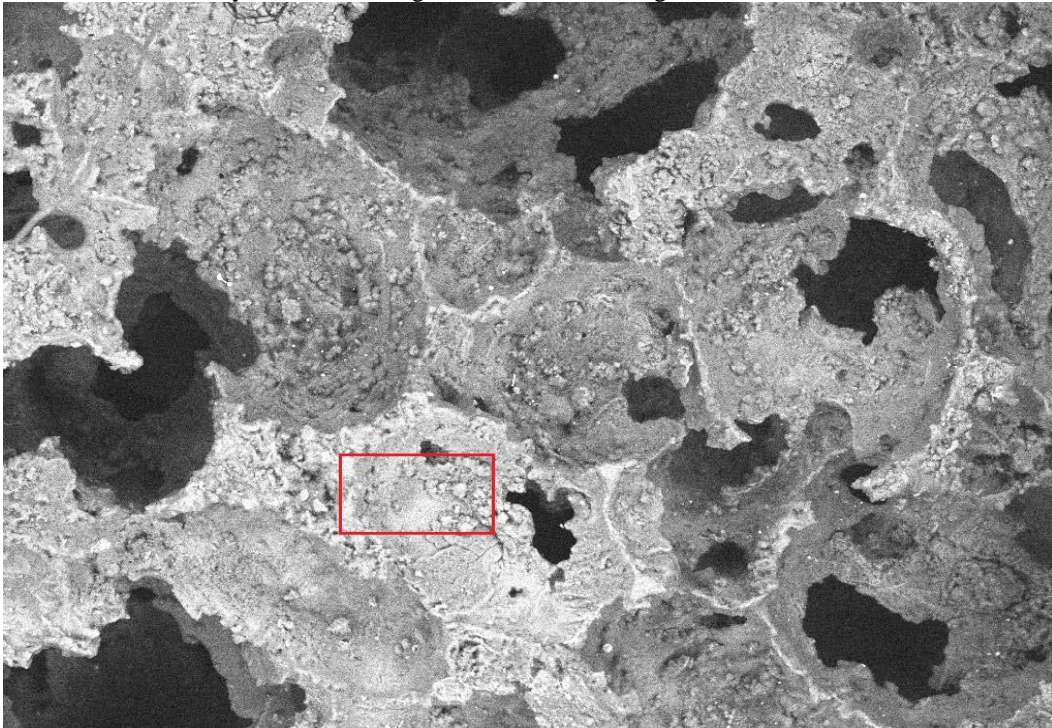
Fig.7 SEM images of cell walls of the aluminum foam with 5 % CaCO 3 and 3% Al 2 O 3 , 45 sec stirring time and 800°C after wire cutting.
